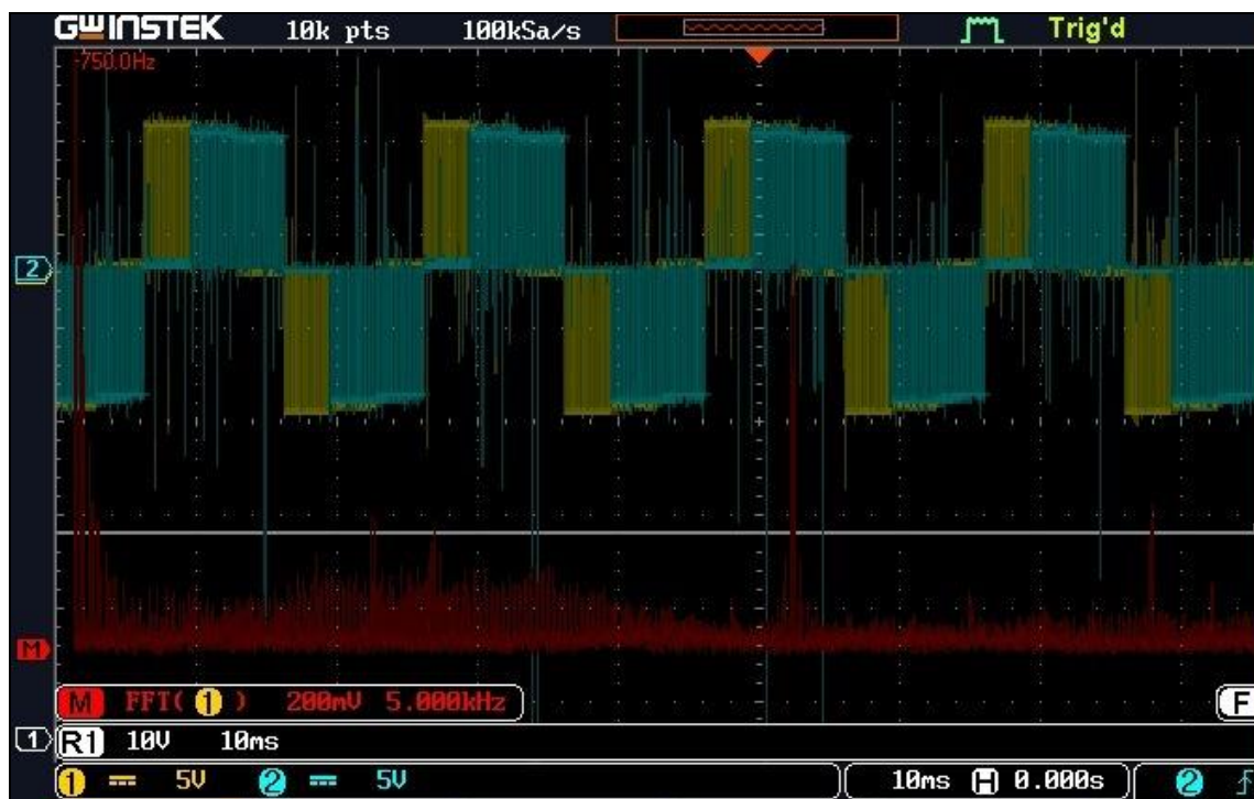
Figure 10: V_{ab} , V_{ac} and FFT for Reference Value 0.8
