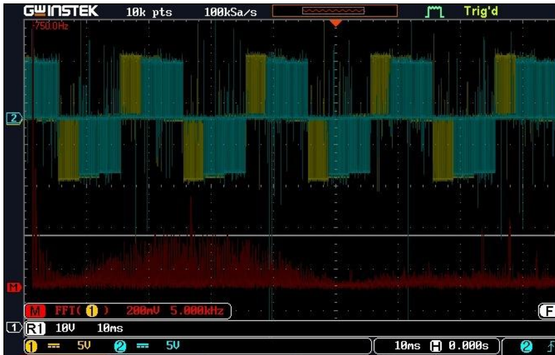
Figure 11: Vab, Vac and FFT for Reference Value 0.5
