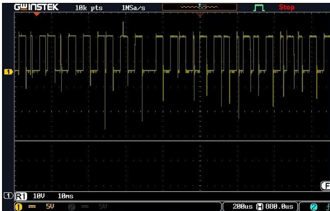
Figure 9: Magnified Phase-Phase Output Voltage Waveform
