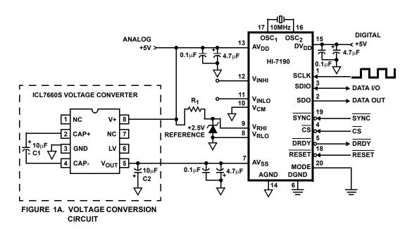
FIGURE 1. SINGLE SUPPLY APPLICATION CIRCUIT
