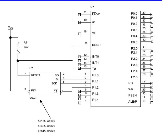
FIGURE 1. INTERFACE OF 8051 TO INTERSIL CPU SUPERVISOR
