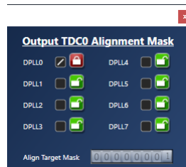
Figure 15. Output TDC0 Alignment Mask for Master
