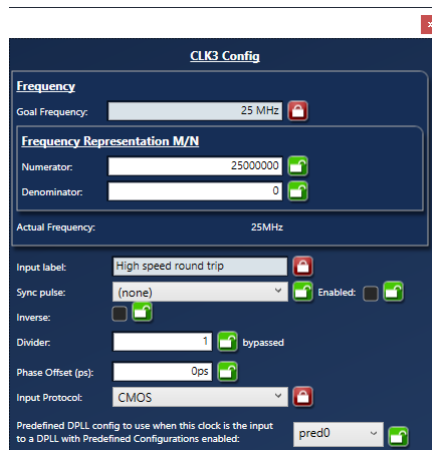
Figure 6. High-Speed Round-Trip Input for Master
