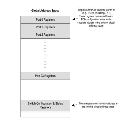
Figure 2 Layout of the Switch's Global Address Space
