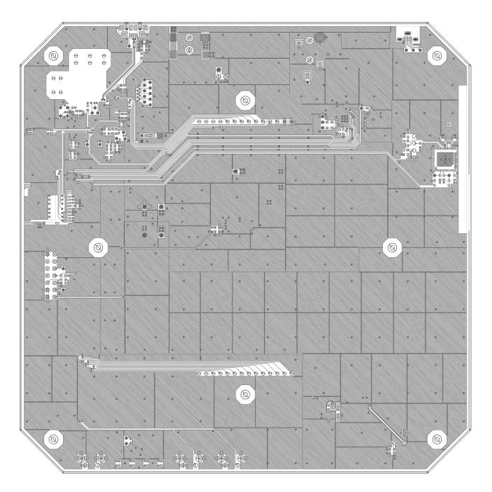
Figure 7-5 4th Layer Pattern (top view)
