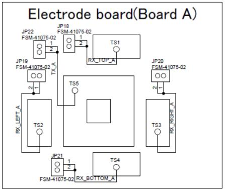
Figure 5-4 Electrode Board Circuit Diagram
