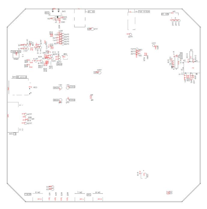
Figure 7-6 Solder Side Silkscreen (top view)
