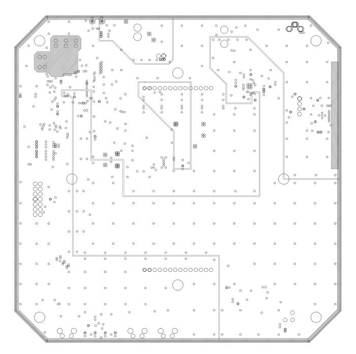
Figure 7-4 3rd Layer Pattern (top view, negative-positive inversion)
