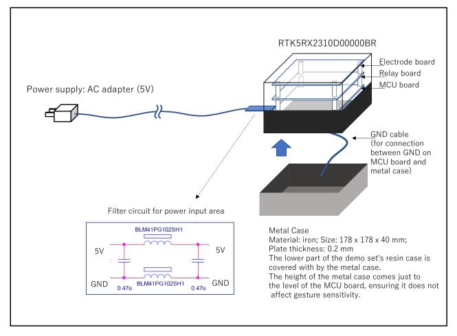
Figure 8-1 EMC Countermeasure Example
