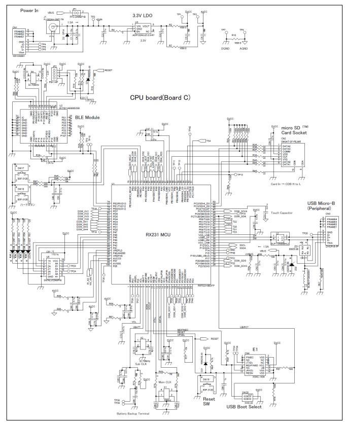
Figure 5-1 CPU Board Circuit Diagram (1/2)
