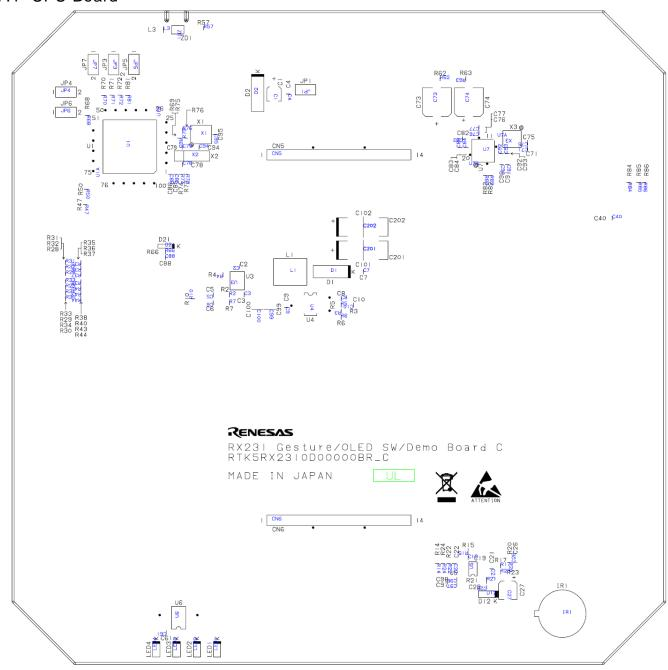
Figure 7-1 Component Side Silkscreen (top view)
