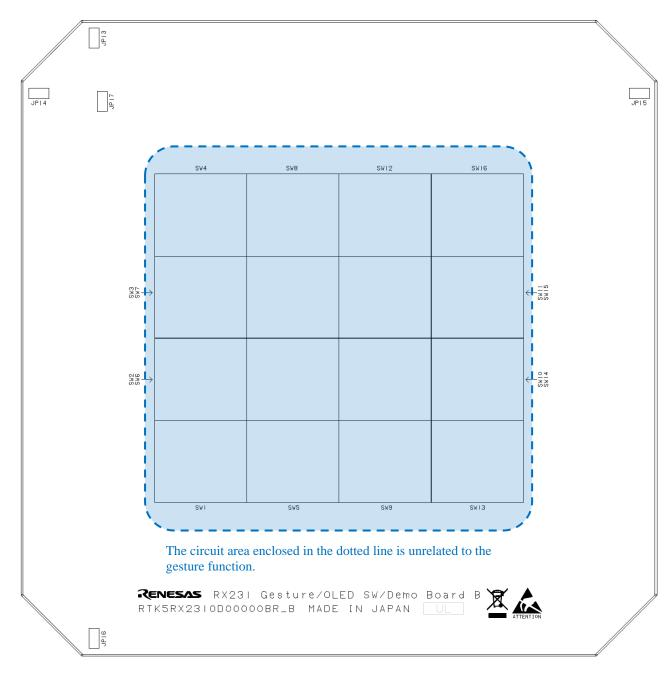
Figure 7-11 Component Side Silkscreen (top view, SW1 to SW16 not used)
