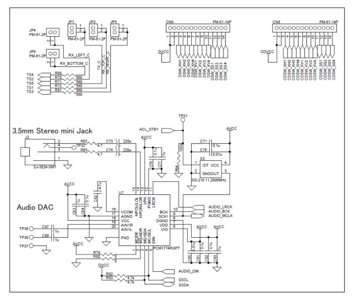
Figure 5-2 CPU Board Circuit Diagram (2/2)
