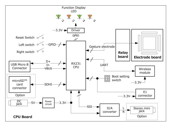
Figure 4-1 Block Diagram
