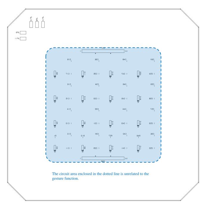
Figure 7-14 Solder Side Silkscreen (top view, jumpers other than JP8 to JP12 are not used)
