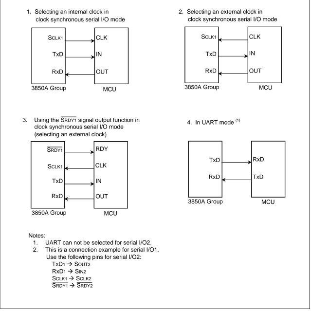
Figure 3.2 Serial I/O Connection Examples (2/2)
