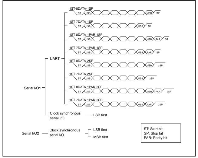
Figure 3.3 Serial I/O Transfer Data Format
