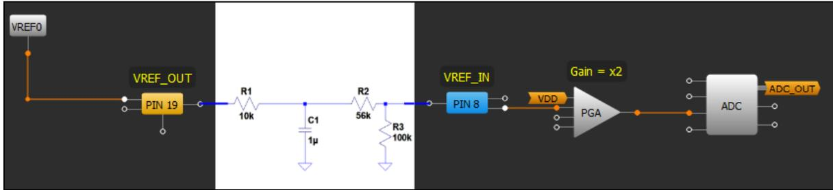
Figure 13. Voltage divider
