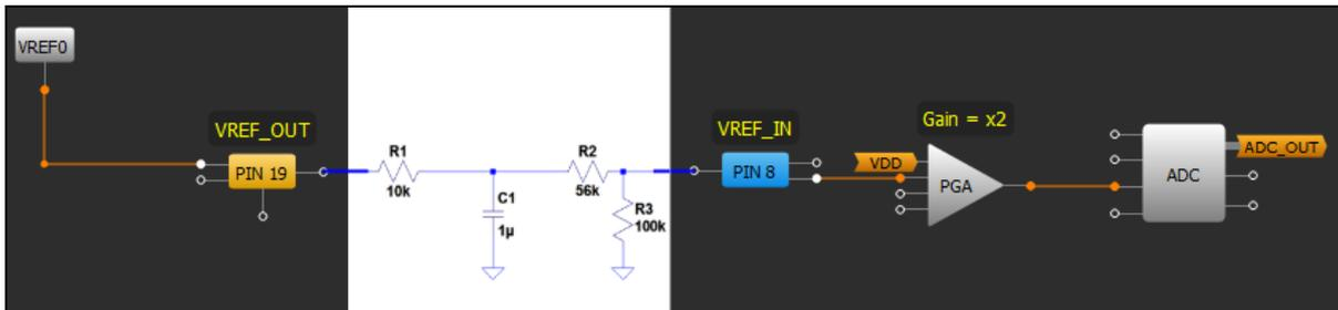
Figure 13 shows how a voltage divider connected to the filter in Figure 8 compensates for this difference. In this case, the PGA gain was set to x2. For simplicity, the resistor voltage divider could be replaced with a potentiometer for small adjustments.
