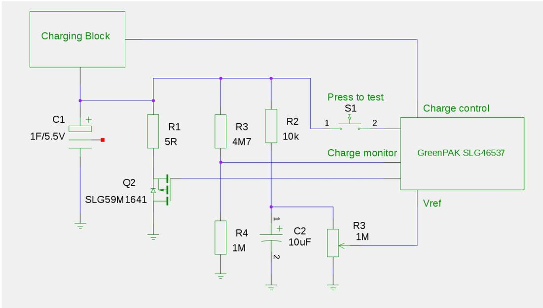
Figure 4. ESR Test – Schematic
