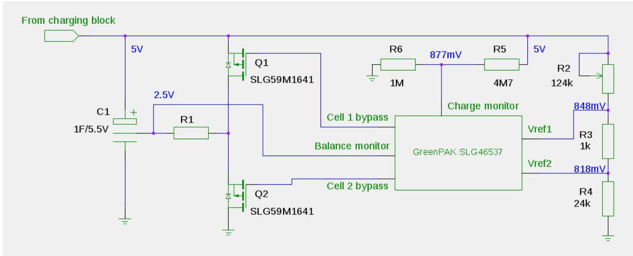
Figure 1. Cell Balancing – Schematic
