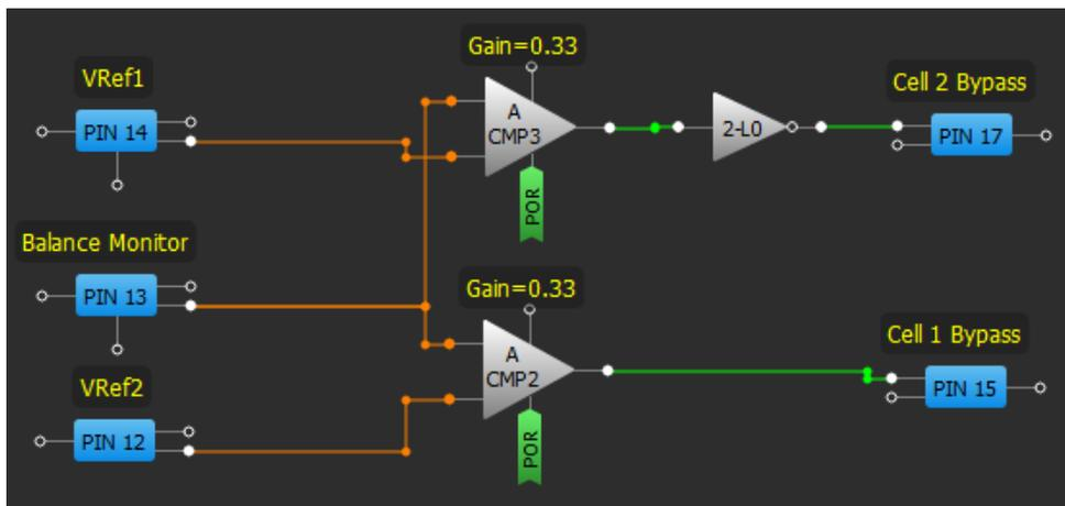
Figure 2. Cell Balancing – GreenPAK Designer Diagram
