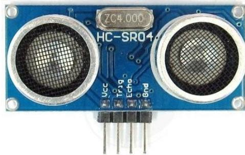
Figure 3. The HC-SR04 ultrasonic sensor
