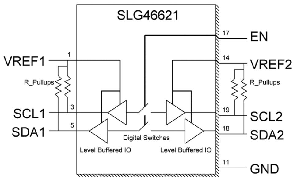
Figure 1. System Level I2C Level-shifter Block Diagram
