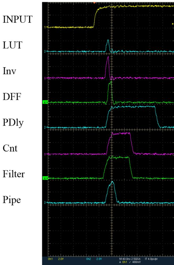
Figure 12. Rising Edge Response Waveforms
