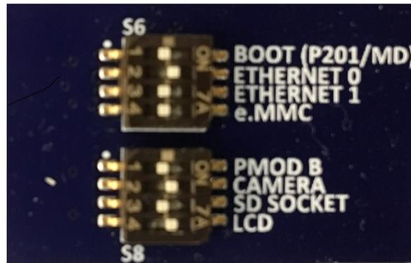
Figure 7. Dip Switch setting for S6 and S8
