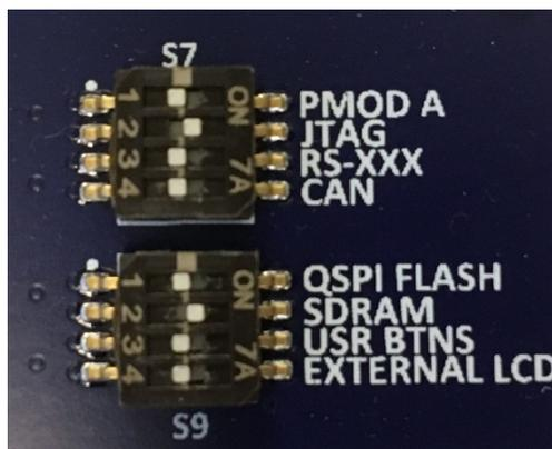
Figure 6. DIP Switch setting for S7 and S9
