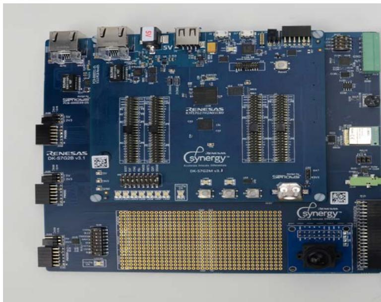
Figure 2. DK-S7G2 connected with Camera Module (OV7670)
