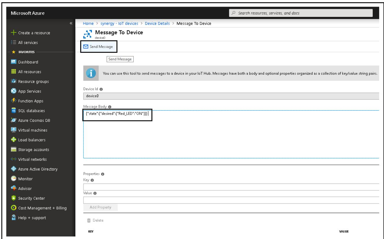
**Figure 47. Snapshot of Send Message to Device from Azure IoT Hub**
