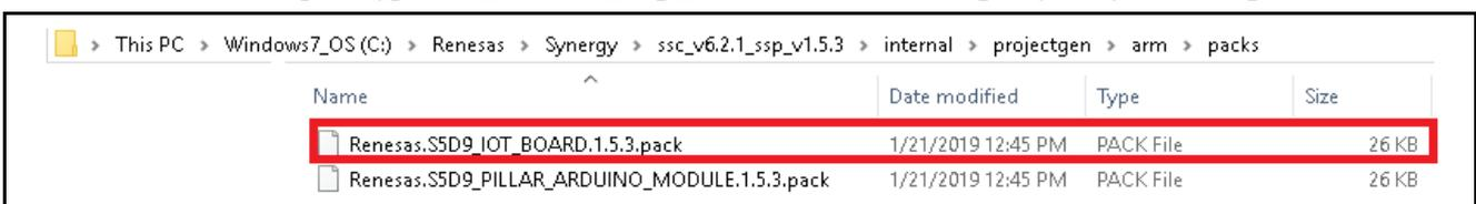
Figure 23. Load BSP Pack for AE-CLOUD1 Kit
