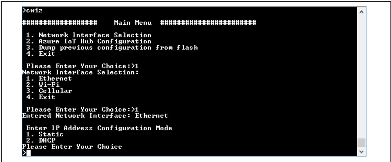
Figure 28. Ethernet Network Interface Configuration Menu
