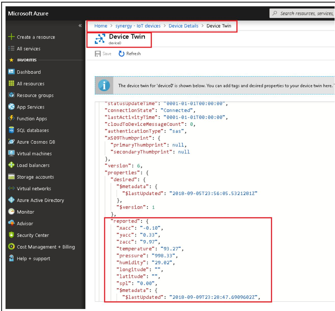
Figure 46. Sensor Data Snapshot on Device Twin
