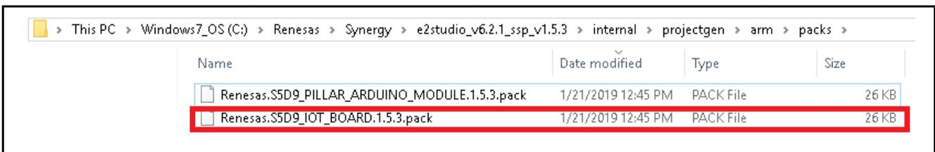
Figure 22. Load BSP Pack for AE-CLOUD1 Kit
