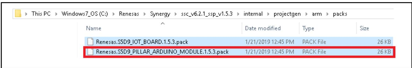
Figure 21. Load BSP Pack for AE-CLOUD2 Kit
