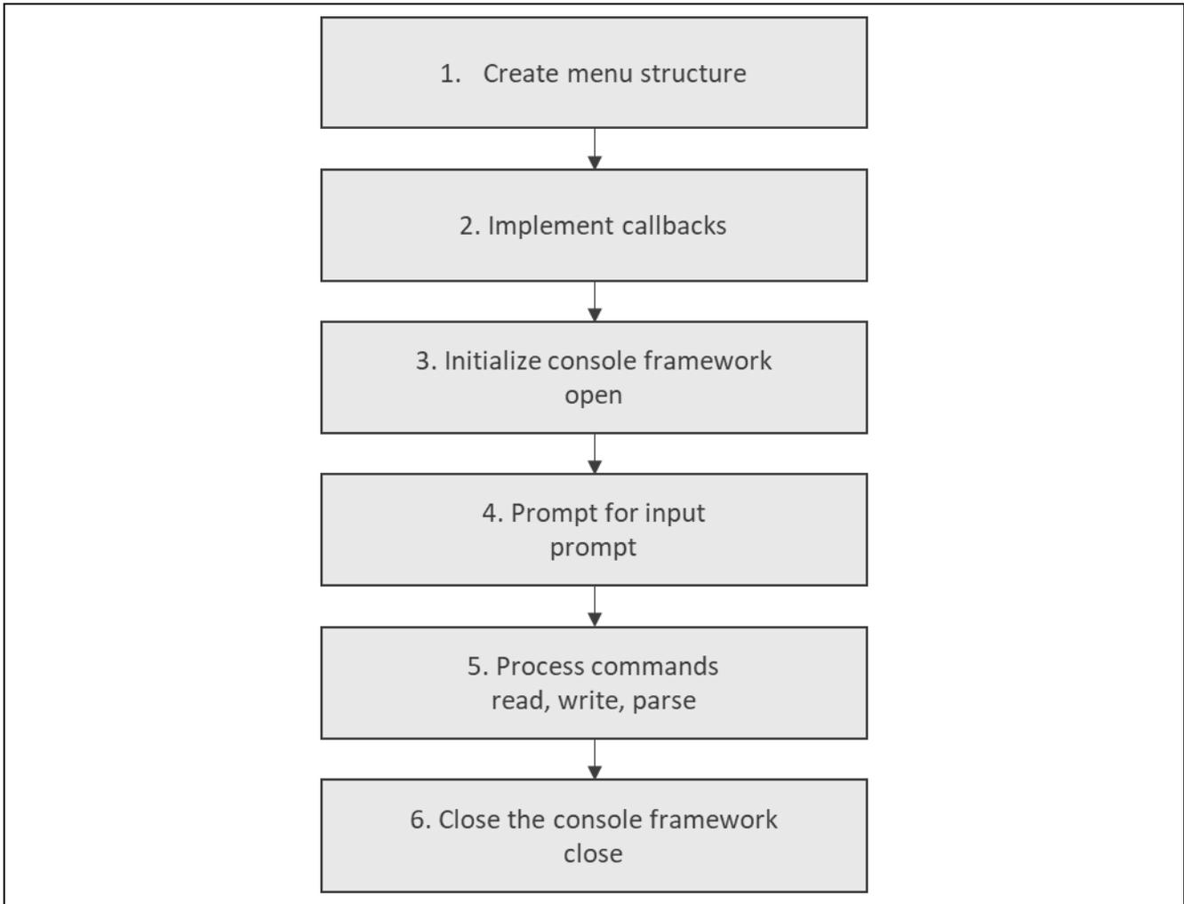
**Figure 6. Typical Console Framework Module Application**
