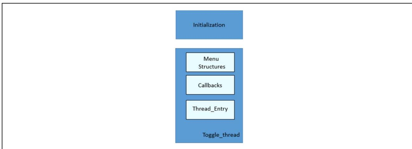
**Figure 8. Console Framework Toggle Command Implementation Block Diagram**
