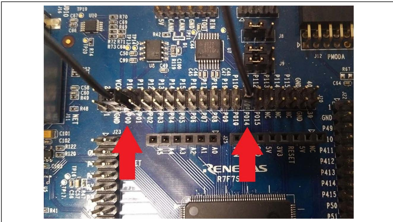
Figure 8 Connecting DAC output pin (P014) with ADC input pin (P00)
