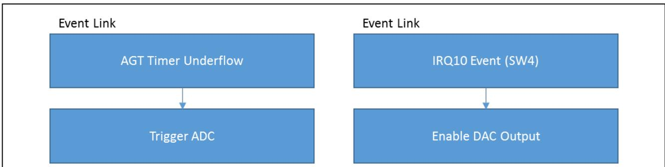
Figure 7 ELC HAL Module Application Project Event Link Diagrams
