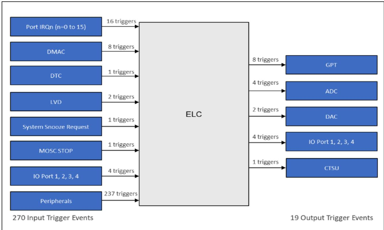
**Figure 2 ELC Hardware Block Diagram**
