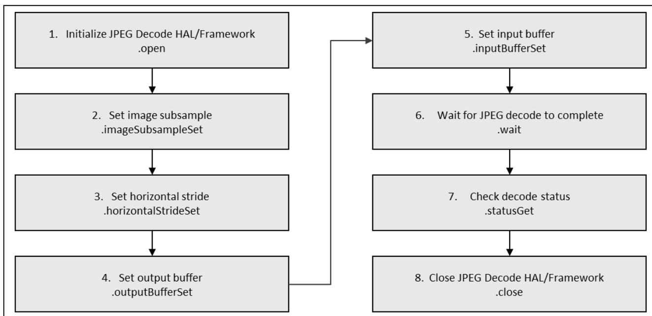
**Figure 3. Flow Diagram of a Typical JPEG HAL/Framework Module Application**
