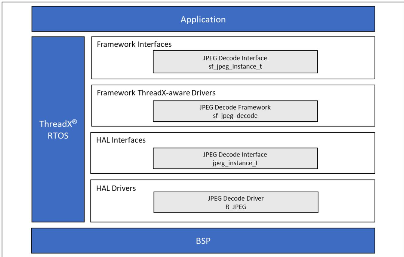
Figure 1. JPEG Decode Framework Module Block Diagram
