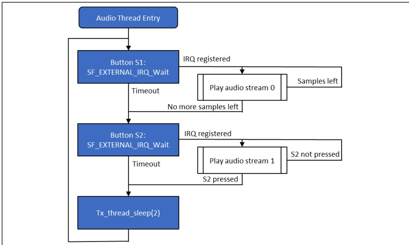
**Figure 9. Simplified audio playback framework processing flow**
