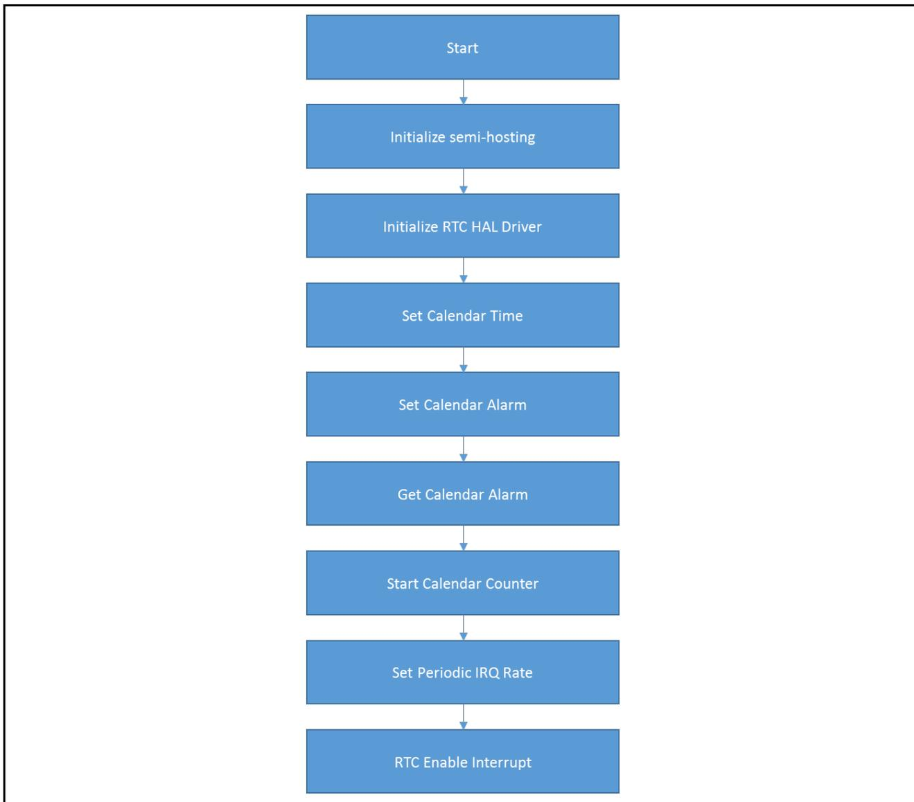
**Figure 5 RTC Application Project Flow Diagram**
