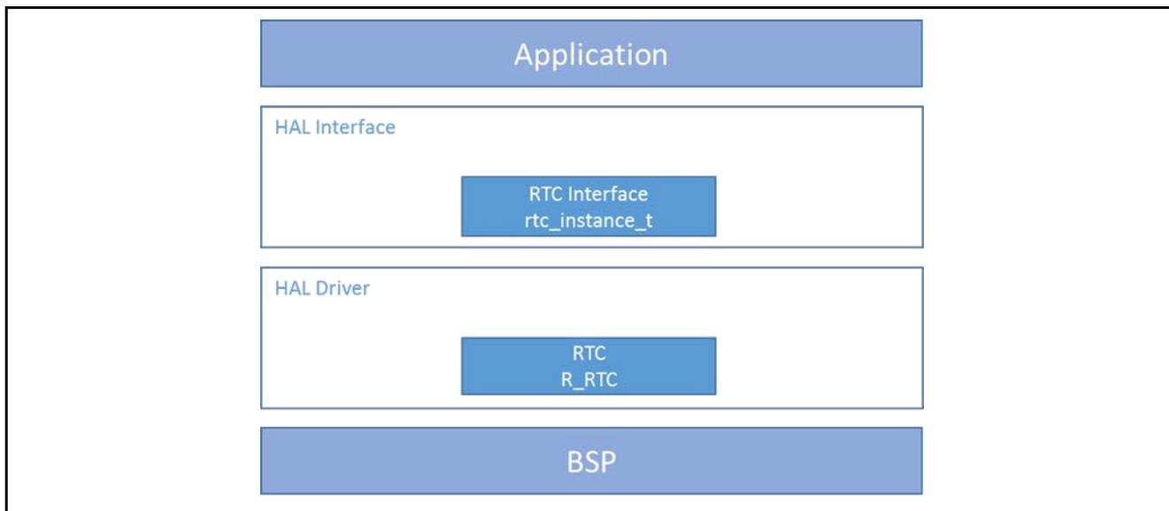
Figure 1. RTC HAL Module Block Diagram
