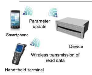
It has been common to use a serial communication interface for such purposes as to update the parameters of a device. In recent years, however, smartphones have come to support Bluetooth Low Energy as a low power wireless interface.
