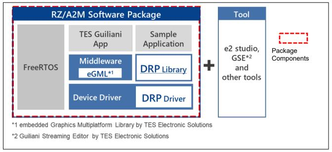
Figure 1 RZ/A2M Software Package Structure
