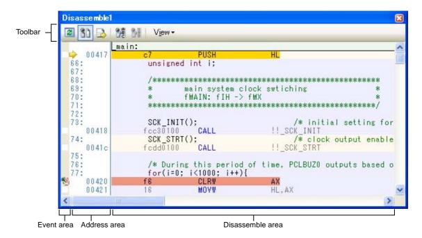
**Remark** You can set the scroll range of the vertical scroll bar on this panel via the Scroll Range Settings dialog box which is opened by clicking the button from [View] on the toolbar.
