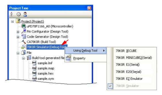
Figure 2-7. Select/Switch Debug Tool to Use
