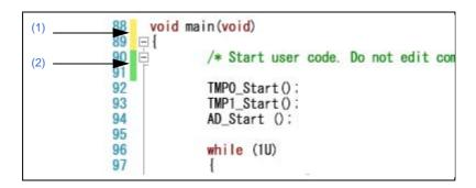
This area changes color only when the downloaded module is out of date (using the "Warning" color of the [General - Font and Color] category of the Option dialog box). This area is valid only when connected to the debug tool and the downloaded source file is opened.
