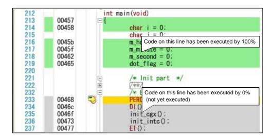
Figure 2-135. View of the Code Coverage Measurement Result (Disassemble Panel)
