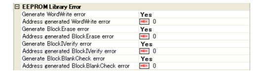
With the properties shown below, specify whether to return error values in the corresponding functions to emulate from the drop-down list (the error values in the functions will not be generated during normal emulation). All properties below are set to [No] by default.
