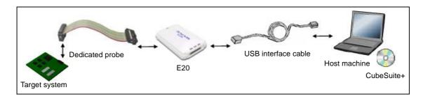
Caution Only serial communications are supported as the communication method with the target system (JTAG communications is not available).
