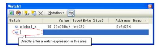
Directly input a watch-expression from the keyboard in the entry box then press the [Enter] key. The input format of the watch-expression is the following tables.
