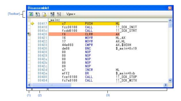
Figure A-21. Disassemble Panel (When Mixed Display Mode Is Not Selected)
