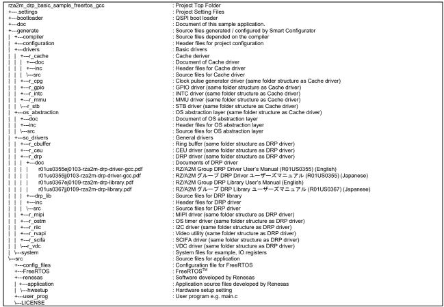
Figure 2.2 Folder Structure of DRP basic sample programs
