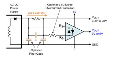
Figure 3. Functional Block Diagram using Optional Filter Capacitors
