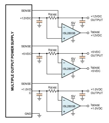
Figure 1. Typical Application Circuit
