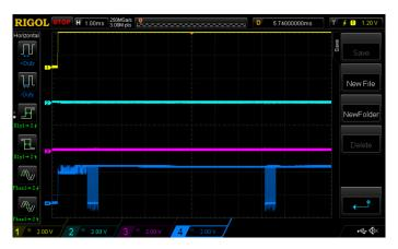
Figure 9. Canon immediate shutter release pattern
