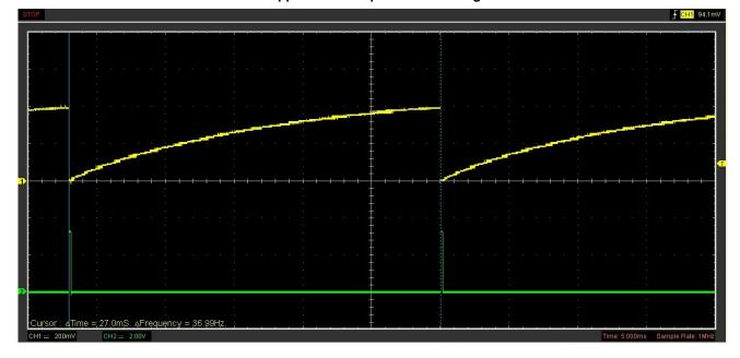
Figure 3. Measured capacitor voltage (Channel 1, in yellow) and output short pulses (Channel 2, in green) for 2
