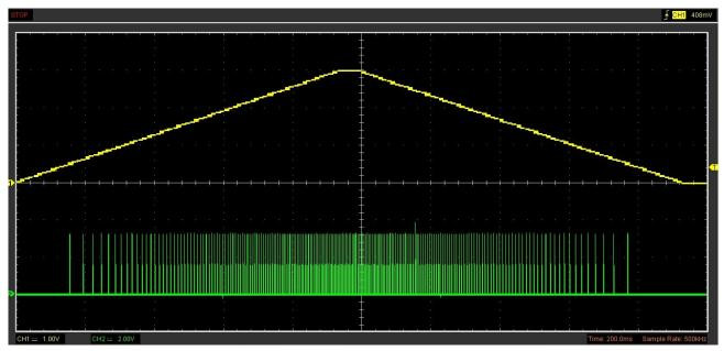
Figure 5. Output signal frequency (Channel 2 in green) in the function of the trapezoidal input voltage (Channel 1 in yellow)
