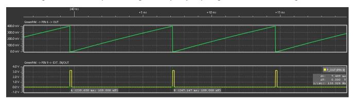
Figure 7. Simulated capacitor voltage and frequency output signal for a DC control voltage of 2V
