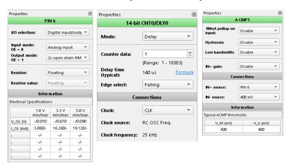
Figure 2. Configuration of PIN 6 as Analog input and Open Drain output, CNT0/DLY0 as Delay element for a falling edge, and ACMP1 configuration
