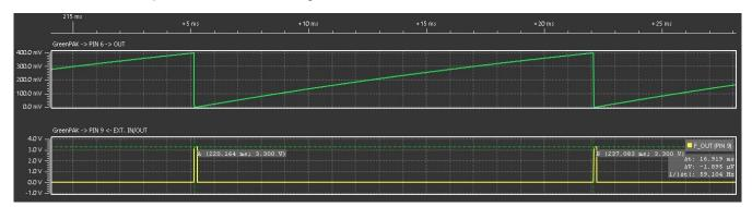
Figure 6. Simulated capacitor voltage and frequency output signal for a DC control voltage of 1V
