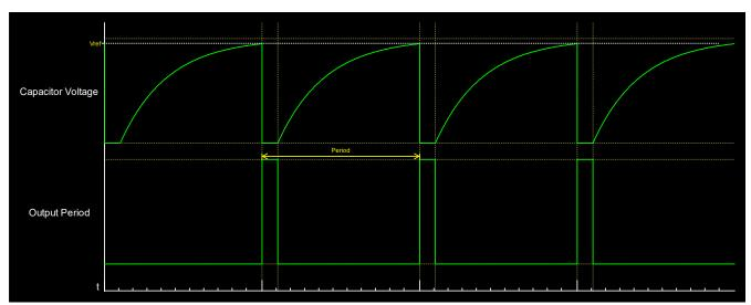
Figure 2. Voltage controlled oscillator circuit operation waveforms
