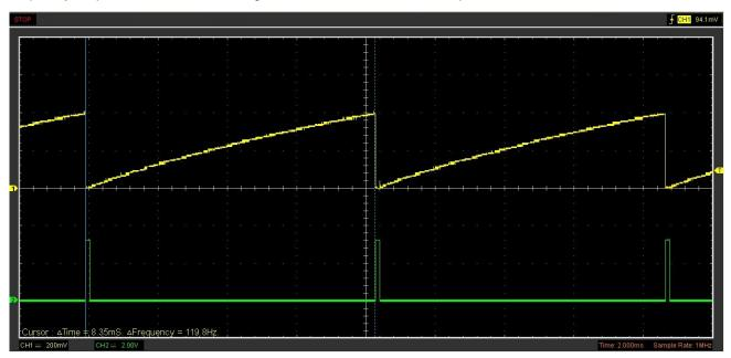
Figure 4. Measured capacitor voltage (Channel 1, in yellow) and output short pulses (Channel 2, in green) for a 1
