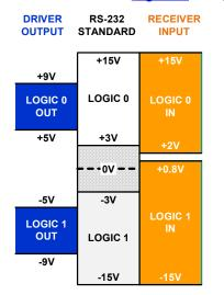
Figure 3. RS-232 Signal Levels
