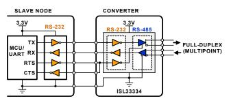
Figure 12. Networking Multiple RS-232 Nodes Through a Full-Duplex RS-485 Link
