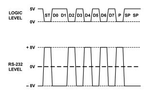
Figure 4. RS-232 Conversion from Logic Signals
