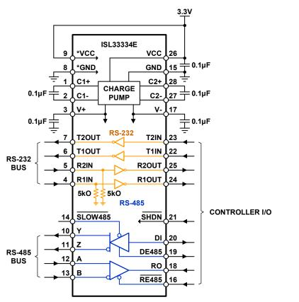
Figure 9. Dual Protocol Transceiver Incorporating One RS-485 and Two RS-232 Transceivers
