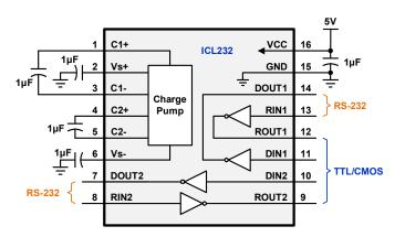
Figure 5. Integrated Transceiver Performing the Signal Conversion
