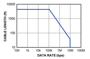
Figure 7. RS-485 Cable Length vs Data Rate Characteristic
