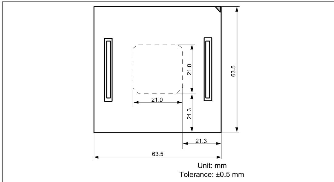
**Figure 7 Dimensions for User System Interface Cable Head**
