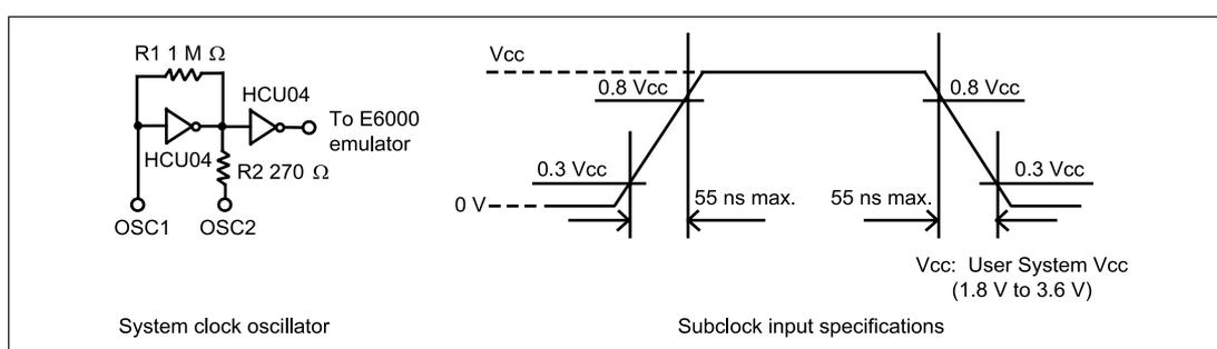
**Figure 12 System Clock Oscillator and Subclock Input Specifications**
