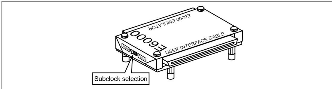
**Figure 9 Expansion I/O board Subclock Selection**
