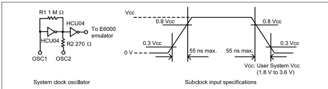
**Figure 11 System Clock Oscillator and Subclock Input Specifications**
