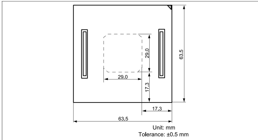
**Figure 6 Dimensions for User System Interface Cable Head**
