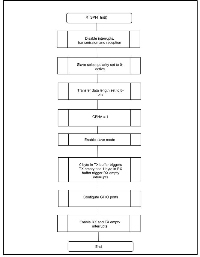
Figure 5-10 Slave Mode SPI Configuration
