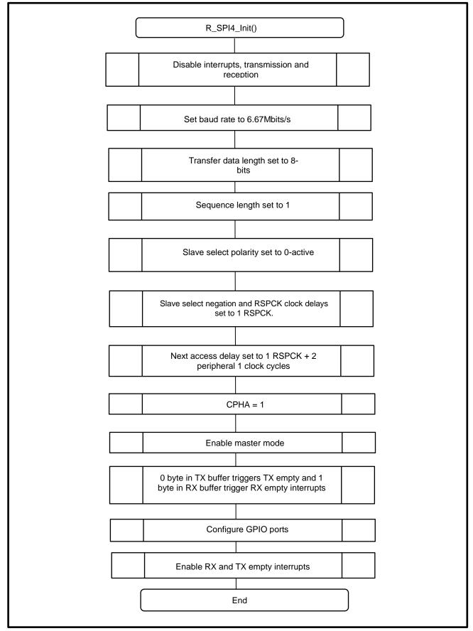
Figure 5-11 Master Mode SPI Configuration
