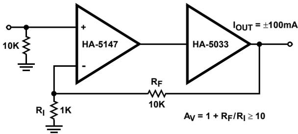
NOTE: The HA-5147's output current can be boosted to  $\pm 100\text{mA}$  by using the HA-5033. AC performance is not affected.
