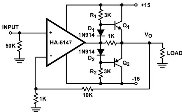
NOTE: The additional drive capability of the power transistors allows the HA-5147 to drive very heavy loads.
