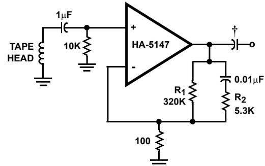
NOTE: This NAB tape playback preamplifier fully utilizes the speed, bandwidth, and noise features of the HA-5147.
