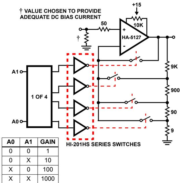
NOTE: Variable gain of 1, 10, 100, 1000 is achieved by selecting the proper amount of feedback with analog switches.
