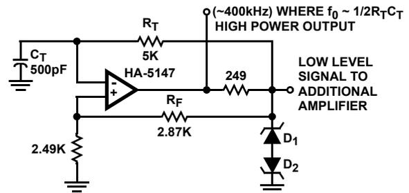
NOTE: Higher frequencies of operation and reduced timing errors make the HA-5147 an attractive building block in signal generation applications.
