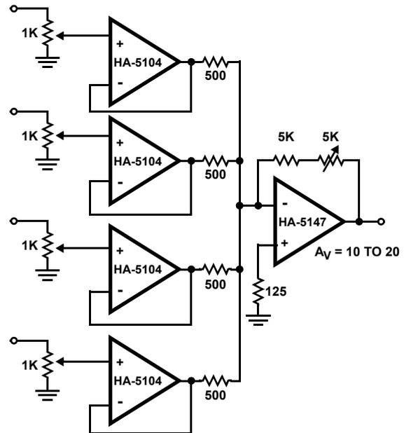
NOTE: Several signals can be combined using this circuit with a minimum of channel crosstalk.
