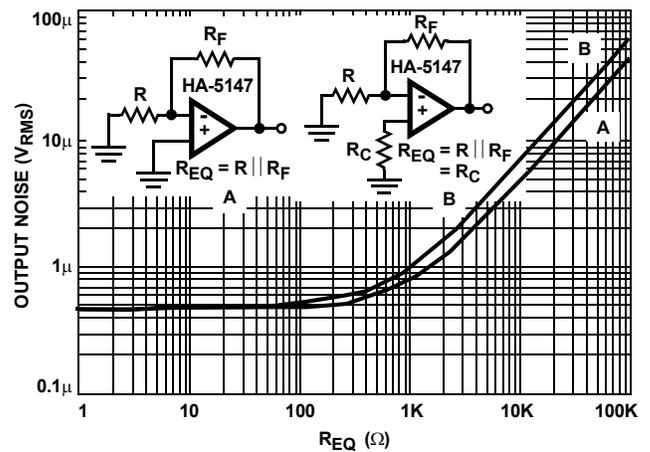
FIGURE 6C. PREDICTED NOISE FOR 10Hz TO 100Hz BANDWIDTH
