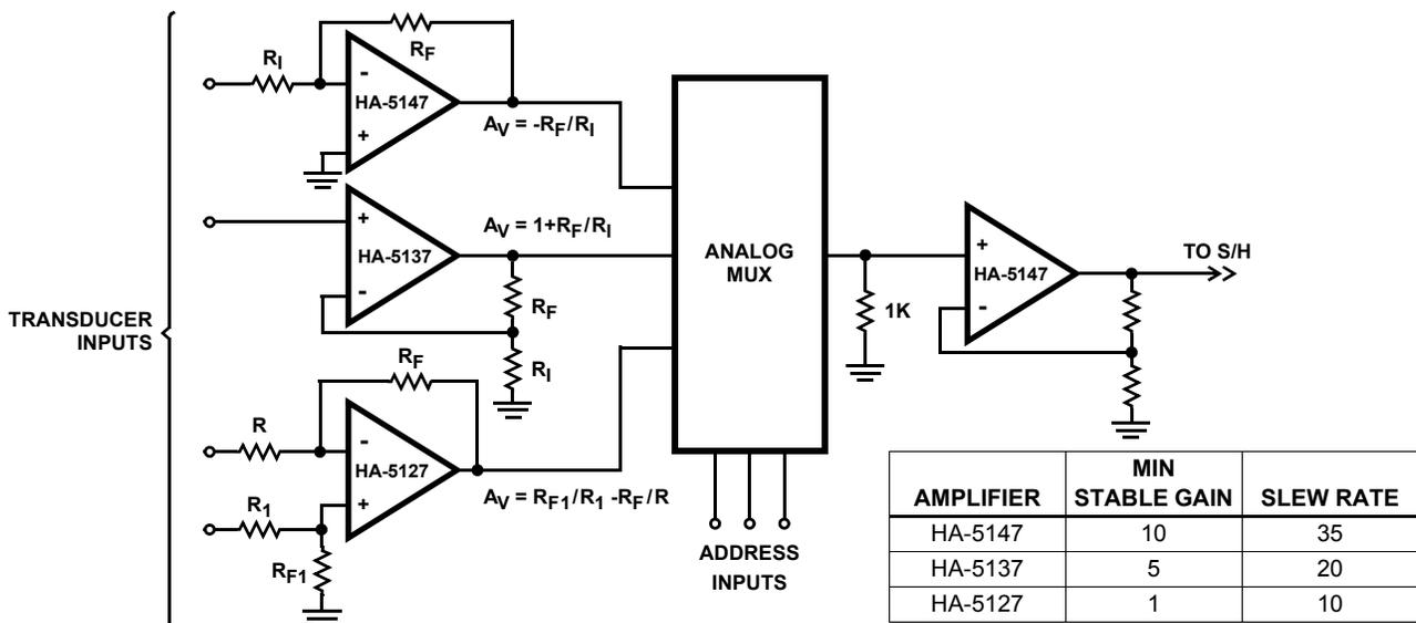
NOTE: Reduced "error budgets" and higher speeds of operation are easily achieved when the combined speed and precision of the HA-51X7 are used in these buffer amplifier applications.
