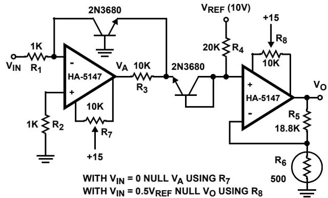
NOTE: The matched pair of transistors makes this a very temperature stable logarithmic amplifier.
