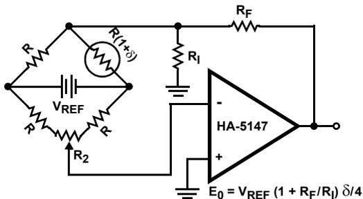
NOTE: Very small bridge signals are sensed and amplified accurately when using the precision performance of the HA-5147.
