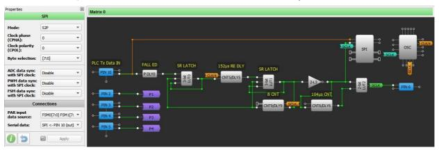
Figure 5. Serial Data from KQ-330F received in SLG46620V
