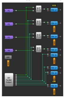
Figure 7. SPI Parallel Output Block Pins
