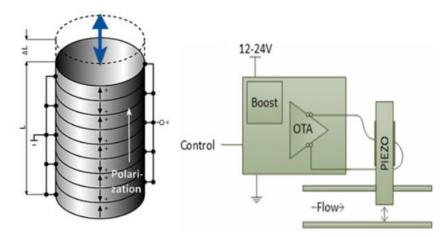
Figure 2: Stacked Piezoelectric device and illustrative drive circuitry
