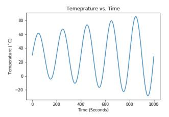
Figure 7: Temperature Vs Time for an unstable controller
