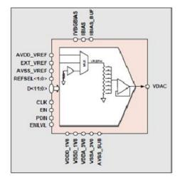
Figure 3: An example of a Renesas 12-bit control DAC IP block
