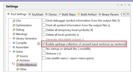
Figure 1 Linker setting for GCC RX
