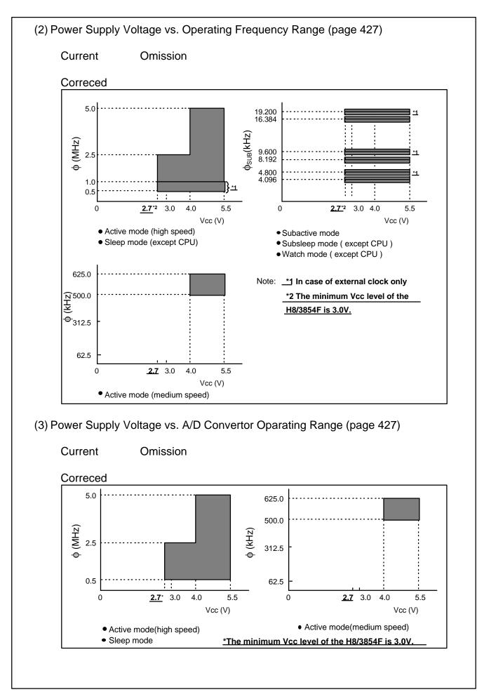
5. In table 16.2 to 16.7(page 428 to 437), the minimum operation voltage (Vcc) is changed from 3.0V to 2.7V for the mask ROM version.
