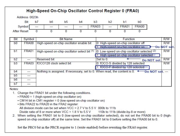
Figure 2-1.High-Speed On-Chip Oscillator Control Register 0 (FRA0) Setting
