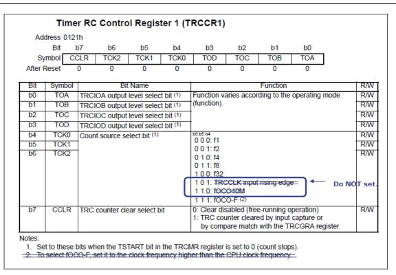
Figure 2-3. Timer RC Control Register 1 (TRCCR1) Setting
