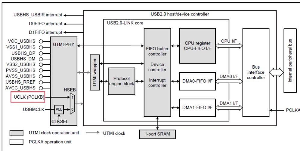
Figure 33.1 USBHS block diagram
