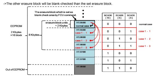
Figure 2 . Example of malfunction (Case1)
