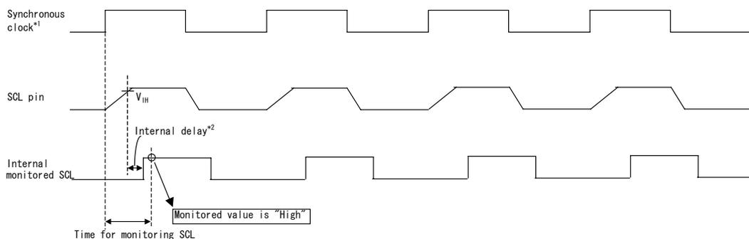
(b) Case that SCL is driven to low by the slave device
