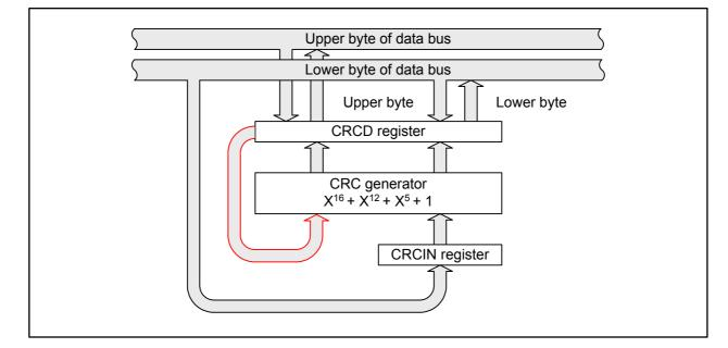
Figure 19.1 CRC Calculator Block Diagram
