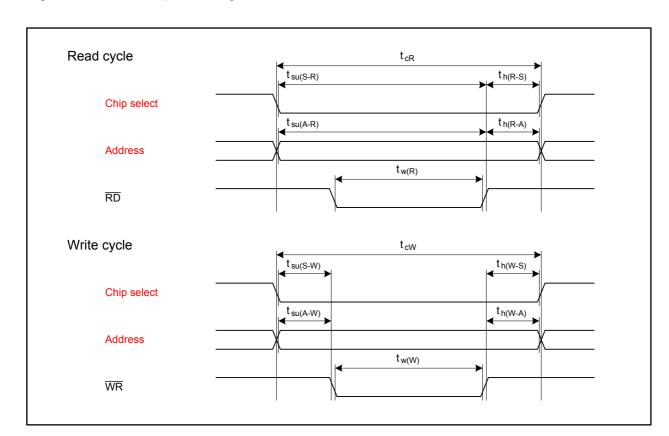
Figure 28.5 Flash Memory CPU Rewrite Mode Timing
