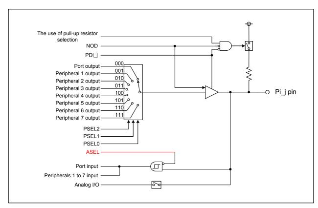
Figure 26.1 Typical I/O Pin Block Diagram (i = 0 to 19; j = 0 to 7)
