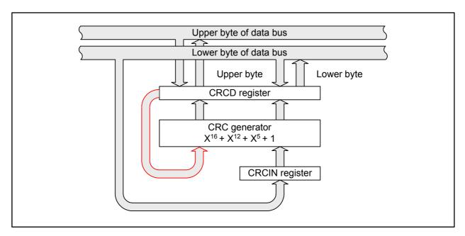
Figure 21.1 CRC Calculator Block Diagram
