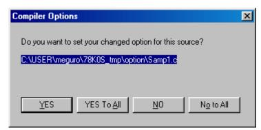
This dialog box is output if a compiler option that is applied to overall files is set while setting filespecific options in the Compiler Options dialog box of PM plus.
