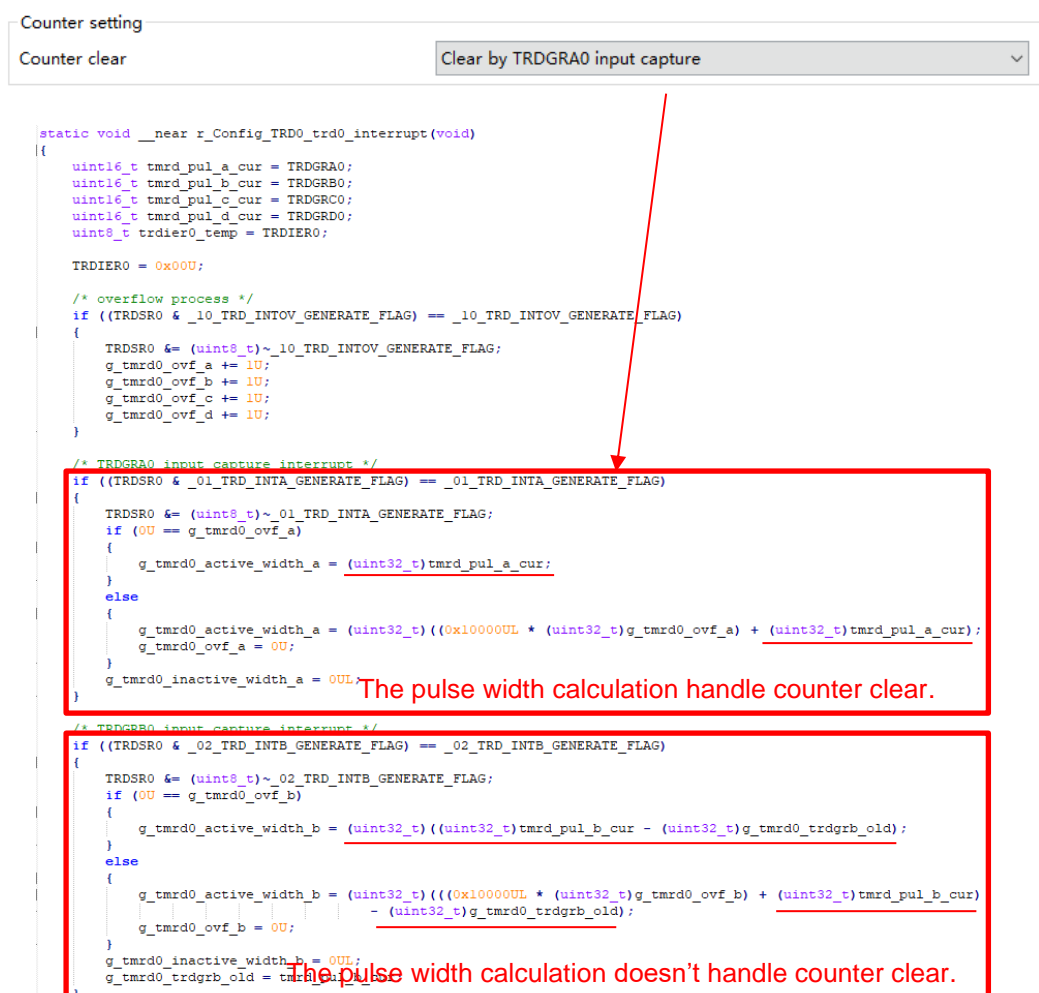
Figure 6-3 Counter clear setting in Input capture function
