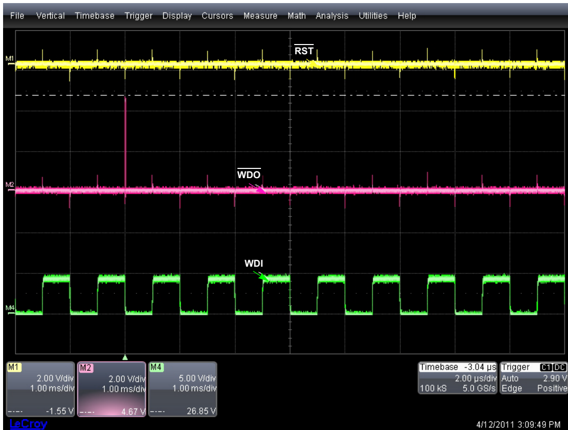
FIGURE 4. TRANSIENT ON \overline{WDO} ( V_{DD} = \overline{MR} = 4.4V , PFI = 1.15V , WDI IS TOGGLING 0 TO V_{DD} AT 1kHz)
