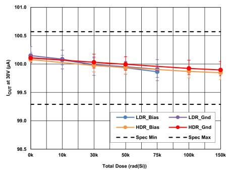
Figure 4. ISL70591SEH output current at 30V ( $I_{O30V}$ ), as a function of total dose irradiation at LDR and at HDR for biased and grounded configurations. The error bars represent the minimum and maximum measured values. The post-irradiation SMD limits are 99.29 $\mu$ A minimum and 100.57 $\mu$ A maximum.
