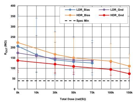
Figure 8. ISL70591SEH output impedance ( $R_{OUT}$ ), as a function of total dose irradiation at LDR and at HDR for biased and grounded configurations. The error bars represent the minimum and maximum measured values. The post-irradiation SMD limit is  $40M\Omega$  minimum.
