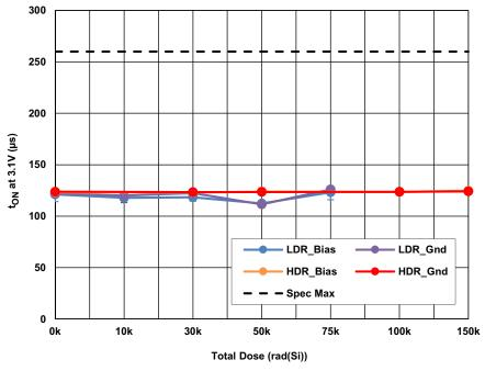
Figure 9. ISL70591SEH turn-on time at 3.1V ( $t_{ON}$ ), as a function of total dose irradiation at LDR and at HDR for biased and grounded configurations. The error bars represent the minimum and maximum measured values. The post-irradiation SMD limit is 260 $\mu$ s maximum.
