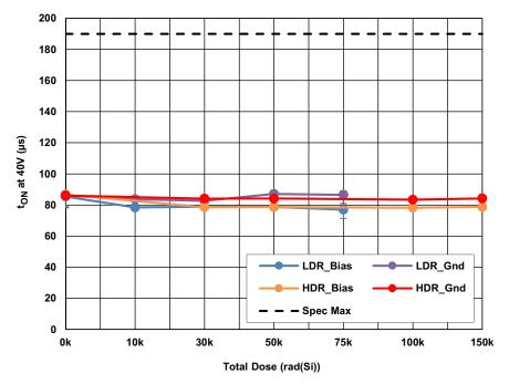
Figure 10. ISL70591SEH turn-on time at 40V ( $t_{ON}$ ), as a function of total dose irradiation at LDR and at HDR for biased and grounded configurations. The error bars represent the minimum and maximum measured values. The post-irradiation SMD limit is 190 $\mu$ s maximum.
