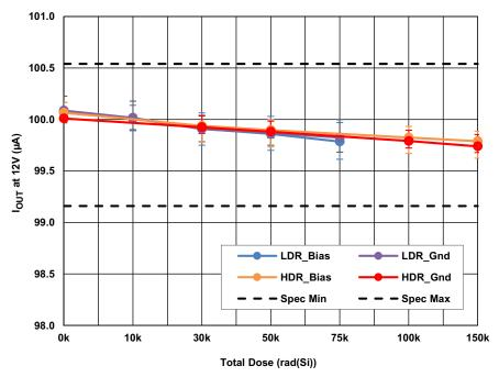
Figure 6. ISL70591SEH output current at 12V (I<sub>O12V</sub>), as a function of total dose irradiation at LDR and at HDR for biased and grounded configurations. The error bars represent the minimum and maximum measured values. The post-irradiation SMD limits are 99.16μA minimum and 100.54μA maximum.
