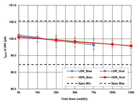
Figure 5. ISL70591SEH output current at 20V ( $I_{O20V}$ ), as a function of total dose irradiation at LDR and at HDR for biased and grounded configurations. The error bars represent the minimum and maximum measured values. The post-irradiation SMD limits are 99.23 $\mu$ A minimum and 100.53 $\mu$ A maximum.
