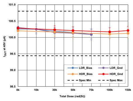
Figure 3. ISL70591SEH output current at 40V ( $I_{O40V}$ ), as a function of total dose irradiation at LDR and at HDR for biased and grounded configurations. The error bars represent the minimum and maximum measured values. The post-irradiation SMD limits are 99.44 $\mu$ A minimum and 100.80 $\mu$ A maximum.
