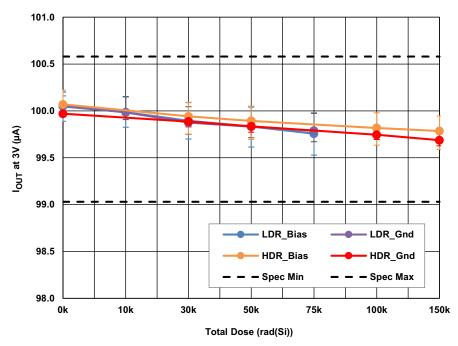
Figure 7. ISL70591SEH output current at 3V ( $I_{O3V}$ ), as a function of total dose irradiation at LDR and at HDR for biased and grounded configurations. The error bars represent the minimum and maximum measured values. The post-irradiation SMD limits are 99.03 $\mu$ A minimum and 100.58 $\mu$ A maximum.
