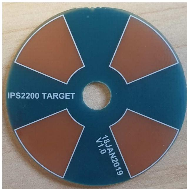
Figure 2. Sensor Target
