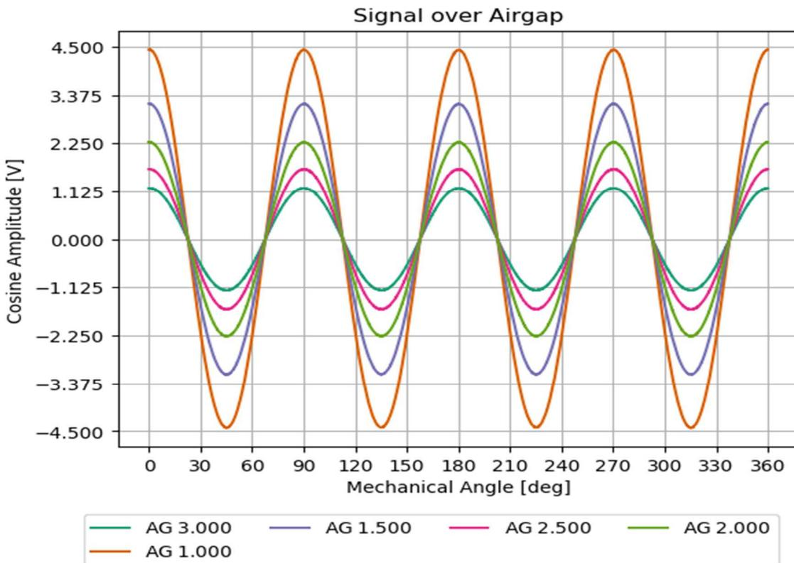
Figure 6. Cosine over Air Gap
