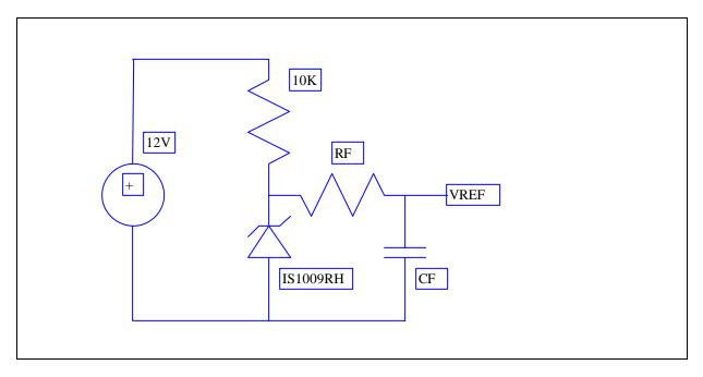
Figure 1: SEE test fixture schematic.
