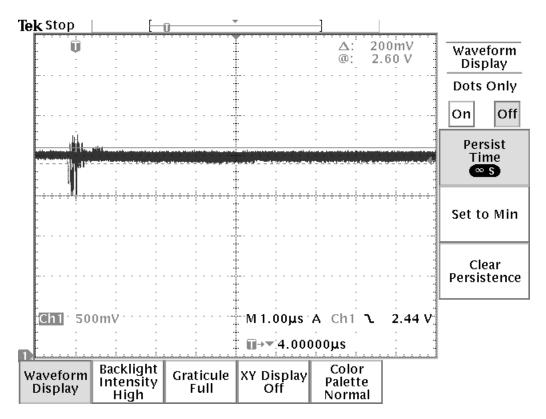
Figure 8: 100uF bypass cap (Ta). 500mV output spikes, capacitor ESR provides limited impulse suppression.
