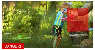
When someone penetrates into a specific area, this system can raise an alert to prevent accident.
