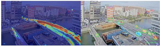
Measuring the moving speed and distribution of target objects (e.g. speed, traffic condition, flow line), visualizes them, and displays alerts.
