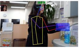
When the particular action is detected in a specific area, this system can raise an alert. In the case of above photo, it detects presence or absence of antisepsis and indicates the status.
