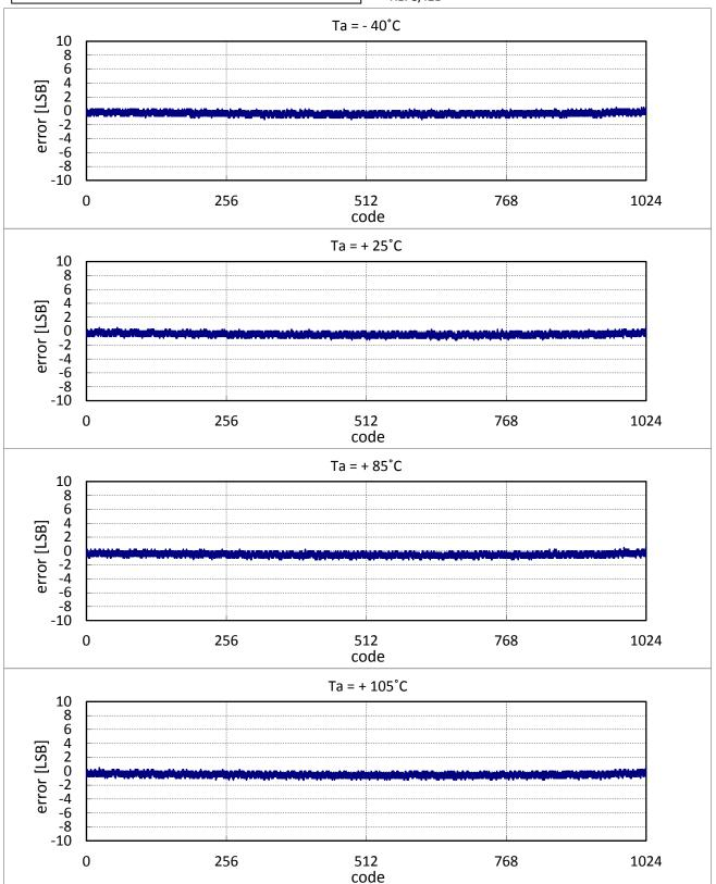
VDD = EVDD0 = EVDD1 = 3.0 V Ta = - 40 °C, +25 °C, +85 °C, +105 °C CPU : LS mode, RUN
