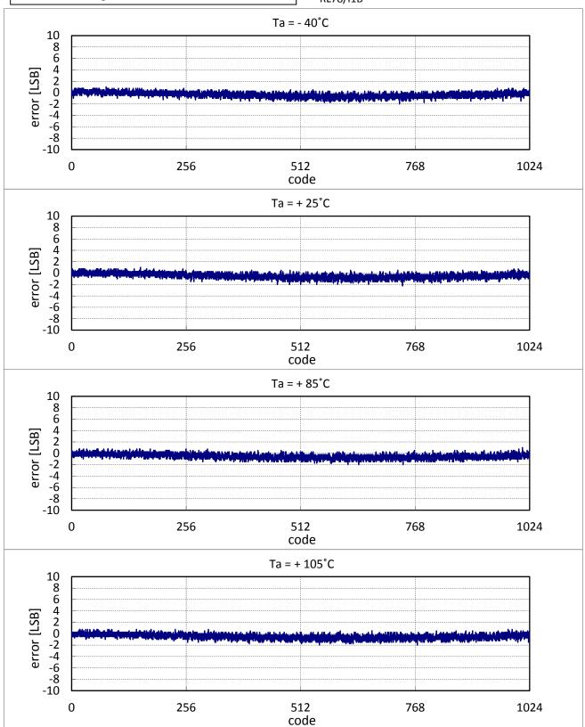
VDD = EVDD0 = EVDD1 = 1.6 V Ta = -40 °C, +25 °C, +85 °C, +105 °C CPU : LV mode, RUN fCLK = 4 MHz (High-speed OCO)
