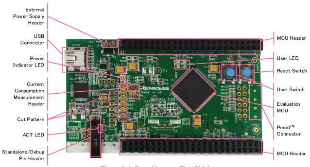
Figure 2-1: Board Layout (Top Side)
