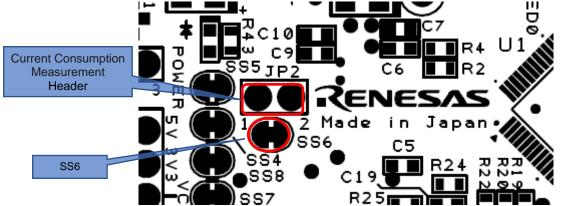
Figure 5-5: Position of Current Consumption Measurement Header and SS6 Cut Pattern
