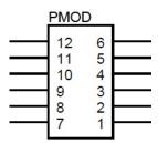
Figure 5-1: Pmod™ Connector Pin Assignment (Top View)
