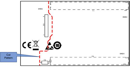
Figure 5-4: Position of Bottom Side Cut Pattern.
