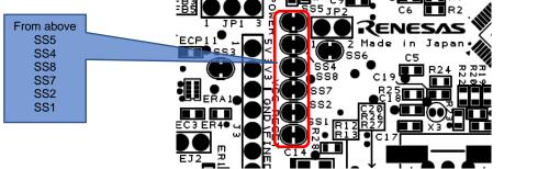
Figure 5-2: Position of Pattern SS1, SS2, SS4, SS5, SS7, SS8
