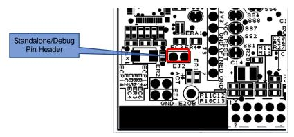
Figure 5-7: Position of Standalone/Debug Pin Header
